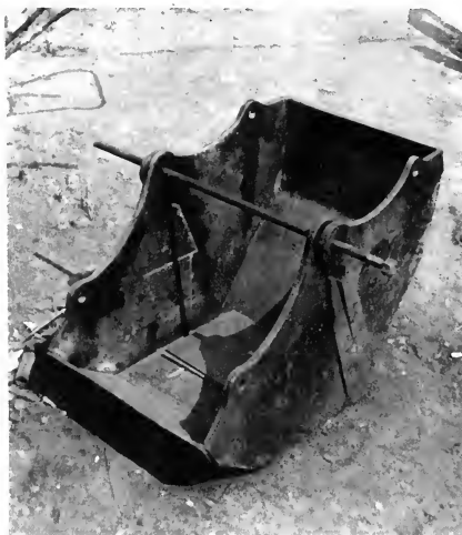
"Clam-shells" are operated by hydraulic mechanism and can be attached to standard back-hoe to clean bog ditches, and perform other useful tasks.
